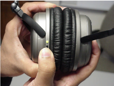
Flip switch to "ON" position to activate ANR; Green indicator light comes on
